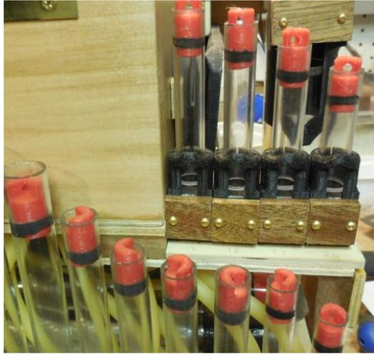
After pipe #1 is tuned, open the door, open the hole #2, and cover the hole #1 with a small piece of masking tape. Close the door. Repeat the procedure. In the same manner, one by one, tune all the pipes.
