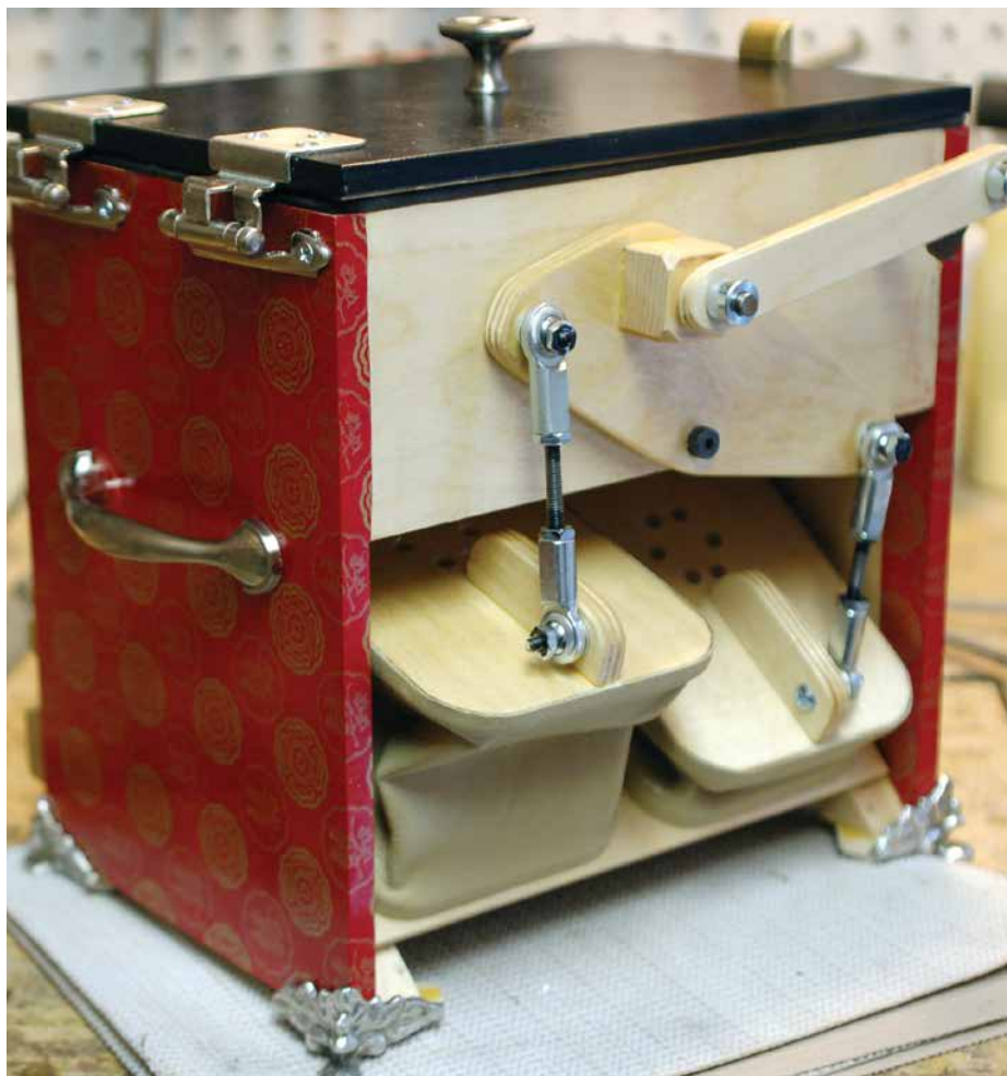
Fig. 5: A view from behind. The rocker that moves two bellows.
