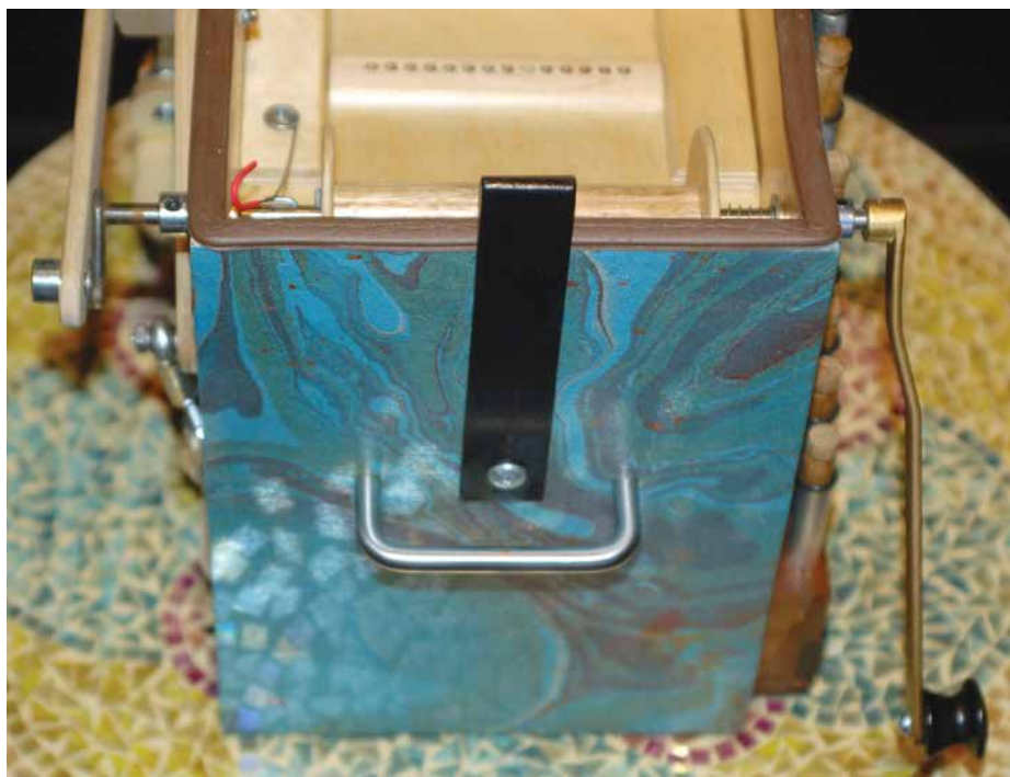
Fig. 6: Spool and crank on a single shaft.
