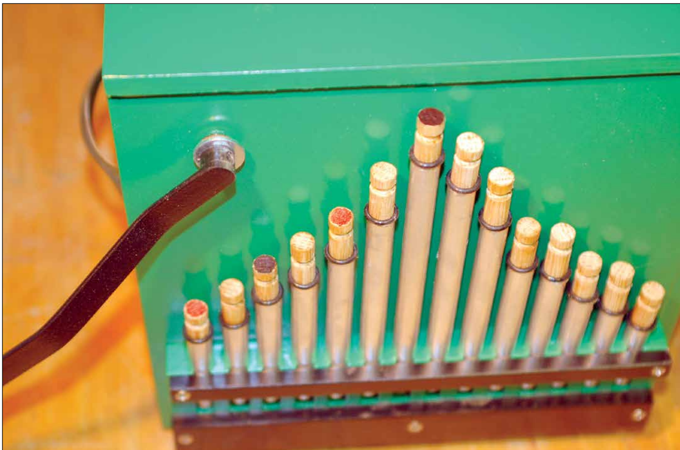
Fig. 2: The C pipes, marked in black, and the G pipes, marked in red, can be tuned up a semitone
