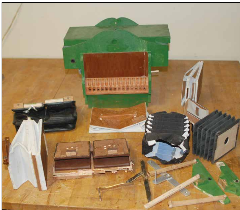
Fig. 4: Several variants of the bellows intended for the MINI-14
