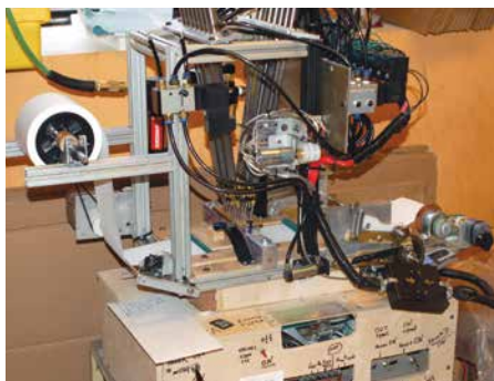
Fig. 7: A pneumatic punch for MINI-14 rolls.
